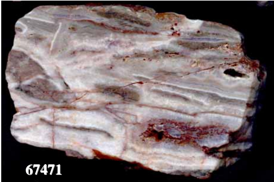
Figure 3: Sample 67471 – Float specimen showing multiple cross-cutting and overprinting crustiform banded quartz veins
