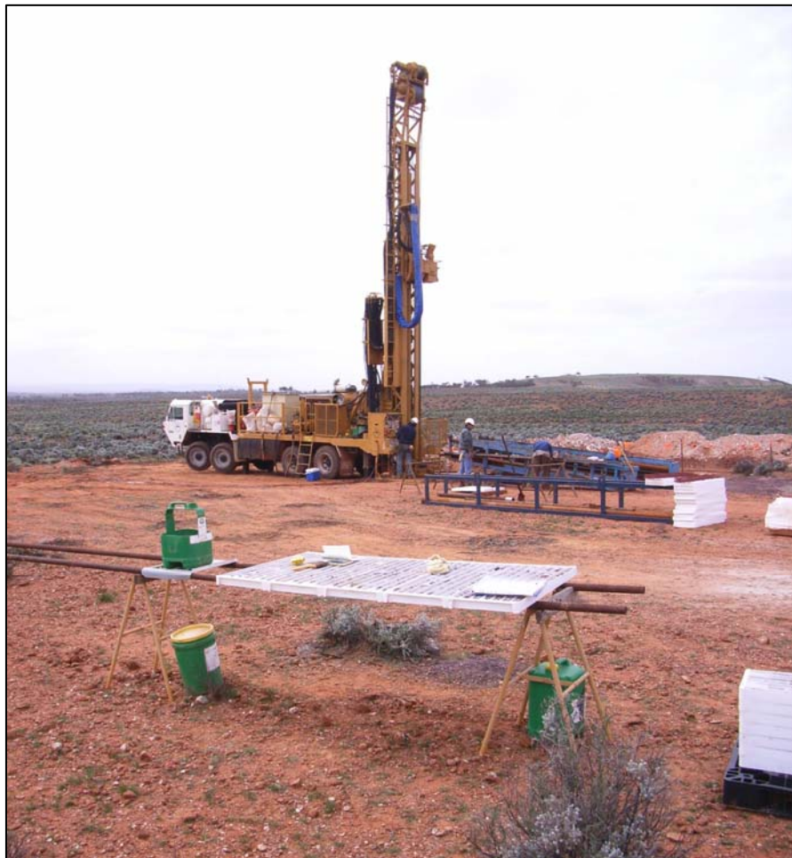
Figure 3: Diamond drilling at Parkinson Dam
