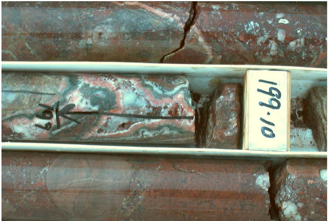
Figure 2: PD 63 drill core, close up photograph of NQ core showing nature of high-grade epithermal veining. (core width 5cm)
