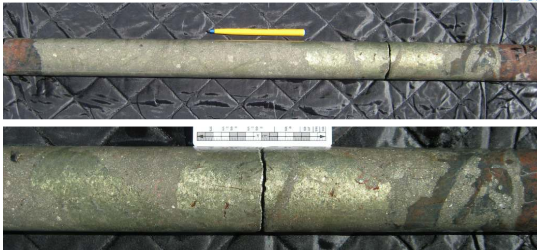
Figure 3: Core photo of massive sulphide interval – pyrite/chalcopyrite. Upper photo 0.65m at 7.82% Cu, 2.41g/t Au. Lower photo detail of this interval.
