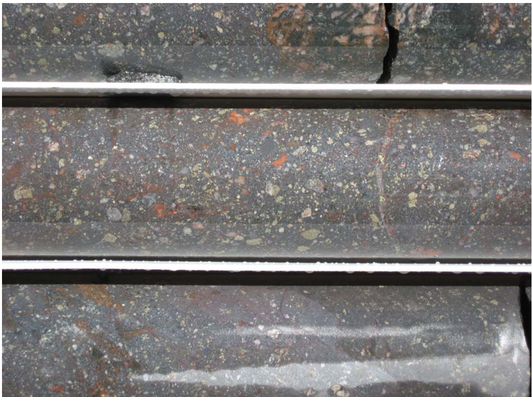
Figure 4: Close-up photo of typical hematite breccia from VUD 7. Hematite is dark grey, sulphides (pyrite and chalcopyrite) are yellow/silverish and the other minerals are carbonate (probably siderite), quartz and feldspar. (NQ Core – approx. 50mm diameter).
